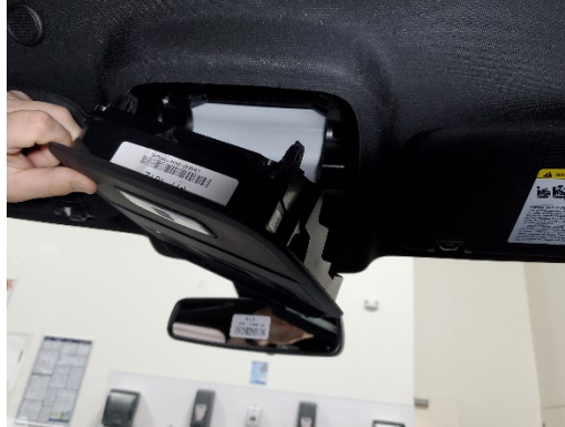
Remove OEM overhead console by gently prying on sides with panel removal tool.
