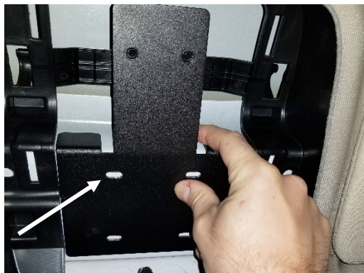
Use backing plate as a template to mark mounting hole locations on OEM metal cross brace.
