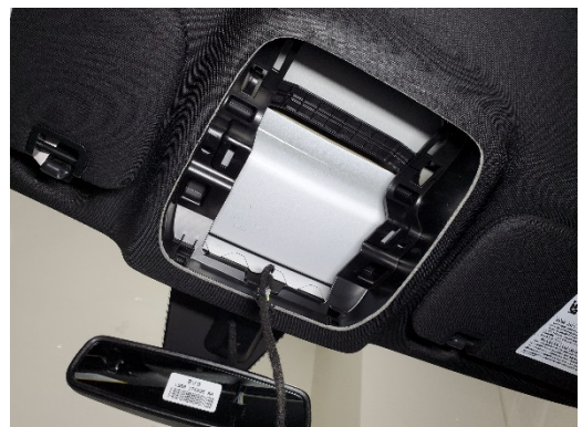
Route necessary wiring at this time through opening in headliner.
