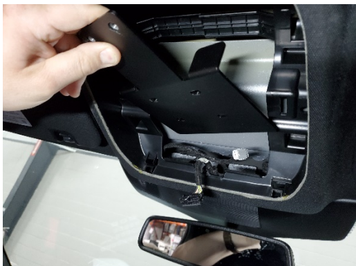
Place backing plate into opening in headliner.
