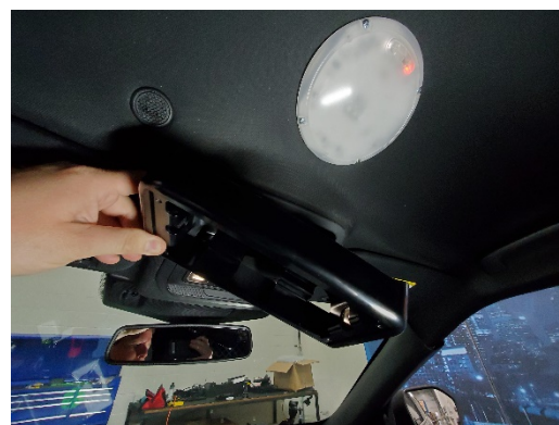
Place new overhead console shroud up to headliner and line up to holes in the backing plate.
