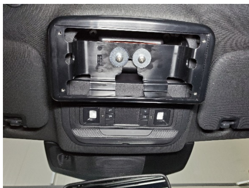
The bolts should be tight enough to compress the lock washers. (Do not over-tighten)
