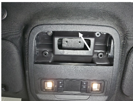
Reinstall OEM overhead center console. Backing plate should be visible through opening.
