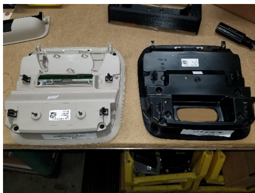
Reattach rear cover to console with previously removed Torx screws. (Explorer and Interceptor Utility shown.)
