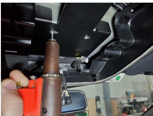
Insert (4) 3/16" rivets into the roof brace.
