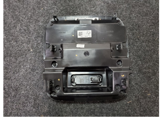
Remove (10) T-20 Torx head screws from rear cover.
