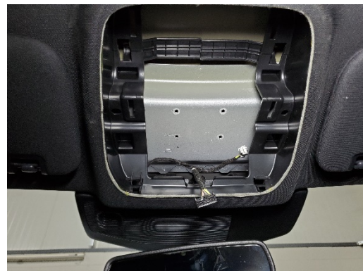
Use 3/16" bit to carefully drill (4) mounting holes in OEM cross brace. Note: Use drill stop to prevent drill bit from touching outer body roof. The metal on the brace is hardened; use of a sharp drill bit is required.
