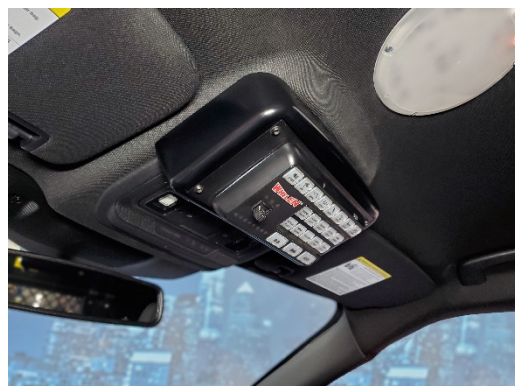
Attach control head to face plate, connect wiring and mount using (4) M4 x 12mm self-threading screws. Installation is now complete
