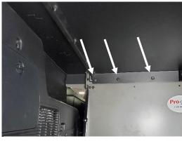
Attach to rear partition using previously removed serrated nuts.
