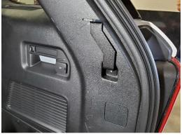
Attach rear-mounting brackets using #8 x 3/4" screws and #8 star washers. Repeat for other side
