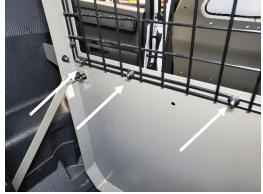
Remove (6) serrated nuts from rear of Pro-Gard partition. Set aside for later step.
