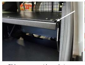
Slide rear support brace between cargo barrier and rear-mounting brackets.
