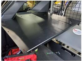
Place driver side, rear cargo barrier into back of vehicle.
