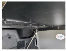
Attach both cargo barrier sides together using 1/4" x 3/4" carriage bolts and nuts.
