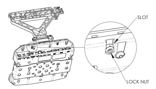
**STEP 3:** WHILE HOLDING LOCK NUT AND SCREEN SUPPORT BRACKET IN PLACE, FASTEN A PAN HEAD SCREW THROUGH MOUNTING HOLE AND LOCK NUT. TORQUE TO 20 IN-LBS ±10%.
