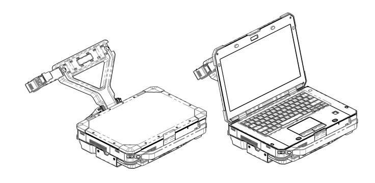
**STEP 6:** ROTATE SCREEN SUPPORT UNTIL CONTACT WITH BACK OF LAPTOP SCREEN.
