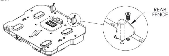
**STEP 2**: ALIGN MOUNTING HOLES OF SCREEN SUPPORT BRACKET WITH MOUNTING HOLES OF DOCKING STATION.
