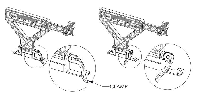
**STEP 8:** RETRACT EXTENSION ARM AND SCREEN HOLDER UNTIL TIGHT FIT WITH LAPTOP SCREEN.
