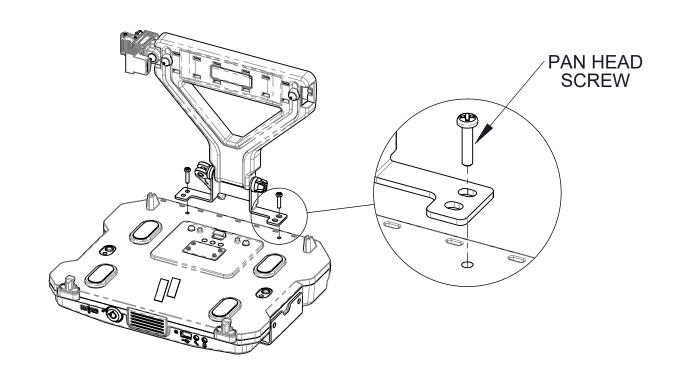
**STEP 4:** REPEAT STEPS 1-3 WITH SECOND LOCK NUT AND PAN HEAD SCREW.
