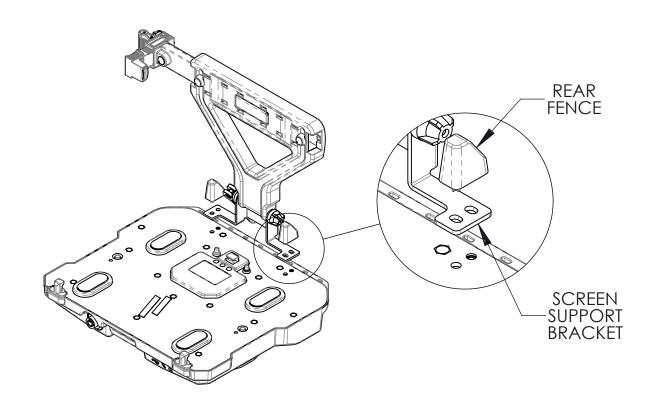
STEP 4: USING A T15 TORX BIT, INSTALL BOTH FLAT HEAD SCREWS THROUGH REAR FENCE, BRACKET, AND INTO DOCK. TORQUE TO 20 IN-LBS  $\pm 10\%$ .
