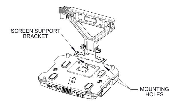
**STEP 2:** POSITION A LOCK NUT WITHIN SLOT BELOW MOUNTING HOLE. ENSURE THAT FLAT SIDE OF LOCK NUT IS FACING INWARDS.
