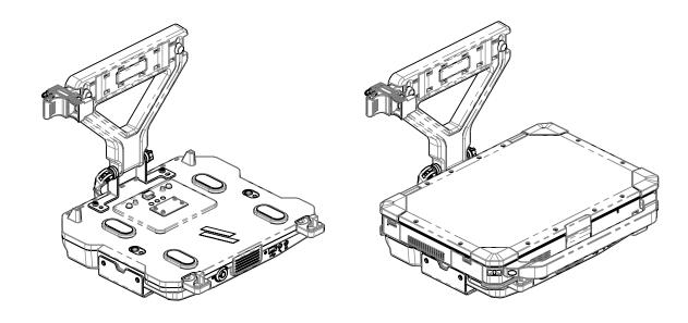
**STEP 2**: EXTEND EXTENSION ARM AND SCREEN HOLDER TO MAX LENGTH WITHOUT REMOVING FROM SLOT.
