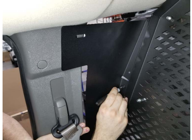
Mark the metal filler mount holes on the Lexan.
