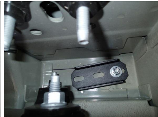
KKM007376 Backing plate and other bulkhead to floor mount hardware shown.
