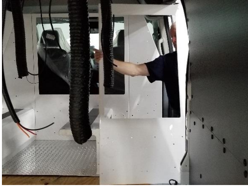
Slide the half bulkhead into the van
