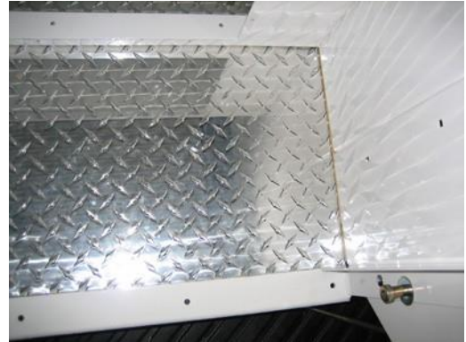
Screw down third compartment door frame with #10 x1-1/4" Phillips screws and install cover over third compartment bench.
