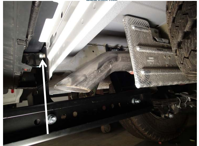
Install passenger side rear bracket (ST006686) with previously removed OEM bolts. Repeat for driver side.
