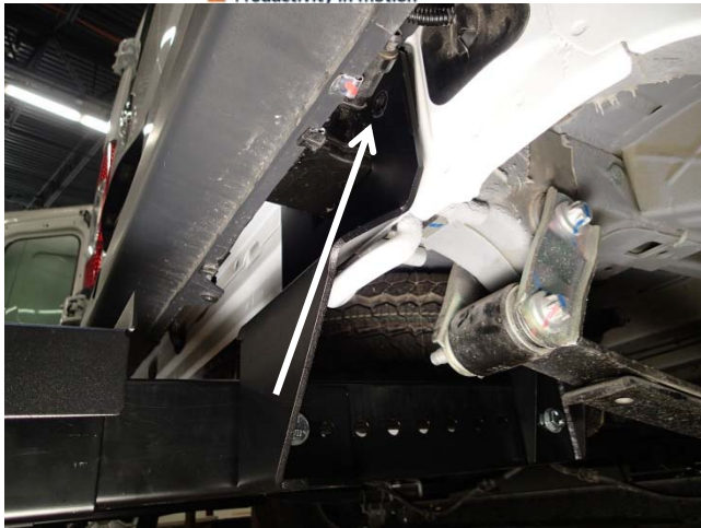
Remove factory bolts located behind OEM rear bumper.
