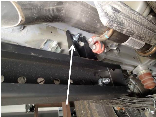
Install front support bracket (ST006439) to driver side frame rail using one (1) 1/2" x 5" bolt, flat washer and nylock nut.
