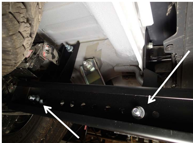
Install support channels to previously installed brackets using two (2) 1/2" x 1.5" bolts, washers, split washers and nuts. (same each side)
