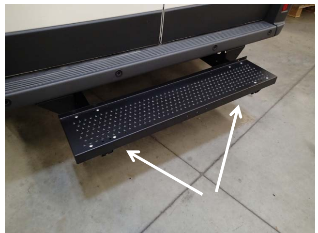
Loosen the eight (8) 1/4" nylock nuts from under the step assembly and slide the step onto the previously installed channel supports using four (4) 1/2"x 3.5" bolts, (8) 1/2" washers and four (4) 1/2" nylock nuts. Tighten all hardware.
