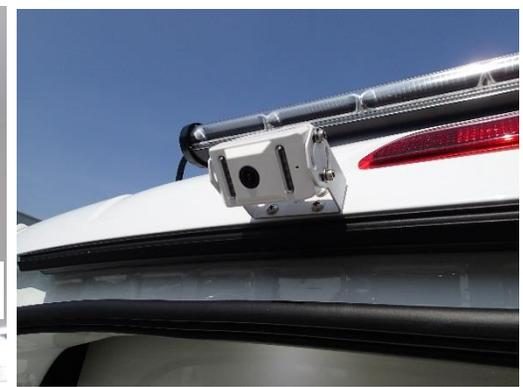
Mount external camera in desired location. If being used for viewing when backing up install camera on backside of roof as close to center as possible. The "U" shape bracket included with camera should work in most applications.
