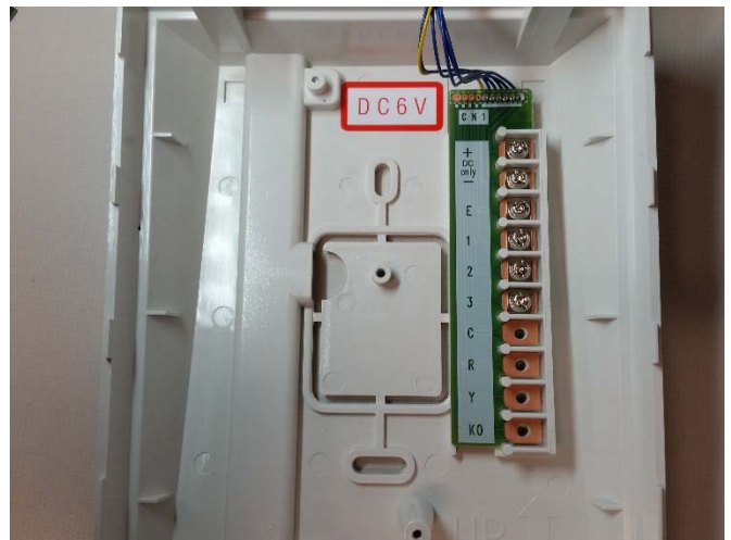
Using the 12 volt to 6 volt DC converter, wire the 6V Intercom Master station following the wiring diagram. The intercom is a 6 volt system and the DC Converter must be used when making power connections.
