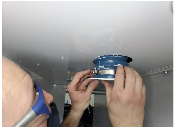
Slide air duct and vent cover into ceiling of kit. Mark and drill 5/32" mount holes
