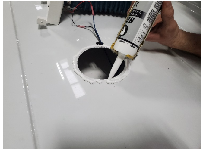
Caulk around holes on vehicle roof.
