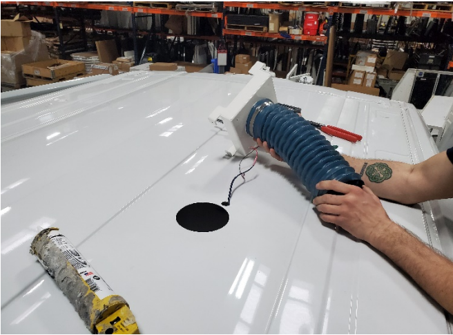
Attach flexible air duct hose to lower vent plate using hose clamp. Insert grommet and connect wiring. (Red - Positive / Black – Ground)
