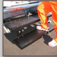
Attaches to rear step for safer entry and exit of the van
