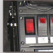
Activates buzzer and warning light when rear compartment doors are open
