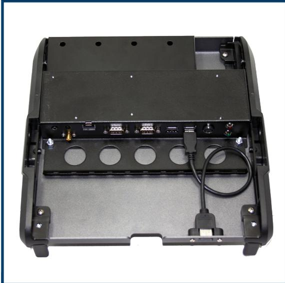
Front facing port replication protects cable connections while integrated strain relief protects from accidental disconnects
