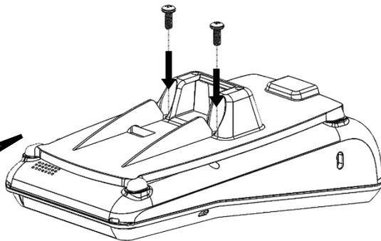
Fit screws supplied and torque to hand tight.
