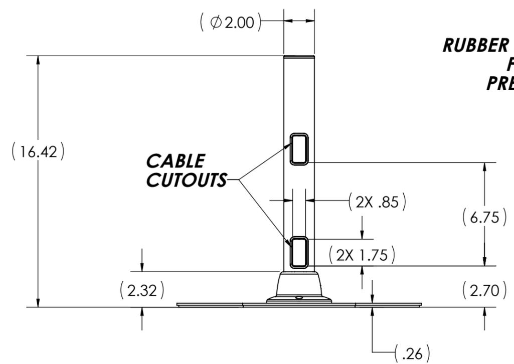
**RUBBER PAD ON BOTTOM OF FREE-STANDING BASE PREVENTS SCRATCHING**
