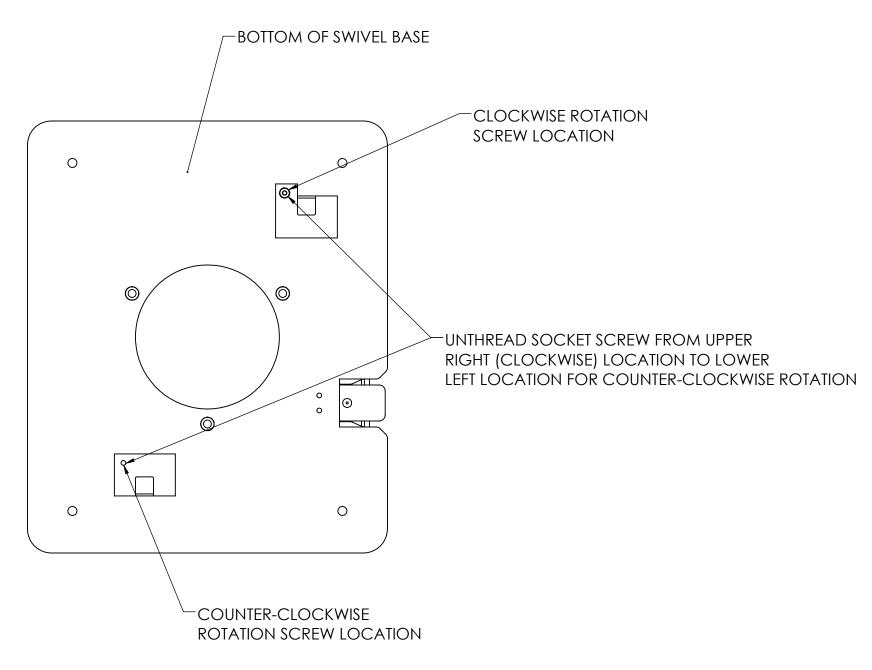
SWIVEL BASE IS ASSEMBLED WITH CLOCKWISE ROTATION FROM THE FACTORY. TO CHANGE FROM CLOCKWISE TO COUNTER-CLOCKWISE, REMOVE ROTATE STOP SCREW AND RE-INSTALL TO COUNTER-CLOCKWISE LOCATION ON BOTTOM OF SWIVEL BASE.
