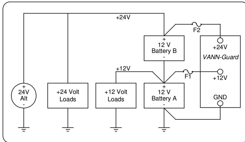
In many 24 volt electrical systems it is desirable to tap into the battery system to obtain power for 12 volt loads. This method, while seemingly simple, causes a charge imbalance resulting in Battery B (see diagram) being overcharged, and possibly boiling, while Battery A discharges.
