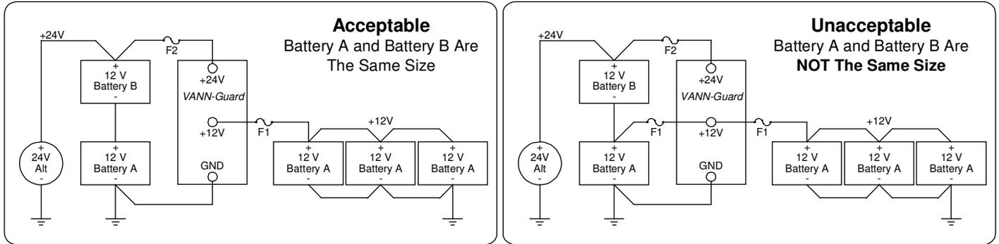
In certain applications, such as private coach or alternate energy applications, it may be desirable to have additional 12 volt “House Batteries” to operate heavy 12 volt (inverter) loads. Use the *VANN-Guard* to charge the additional batteries.
