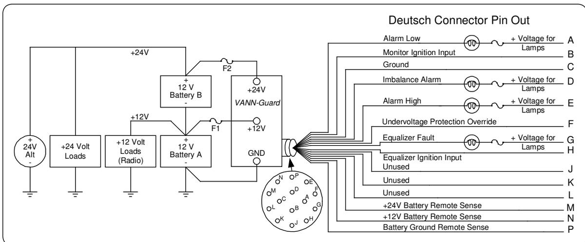
The monitor output from the unit is a through a Deutsch brand connector P/N: HDP20-18-14PN it's mating connector is the Deutsch P/N: HDP26-18-14SN housing with Deutsch P/N: 1062-16-0622 socket contact.
