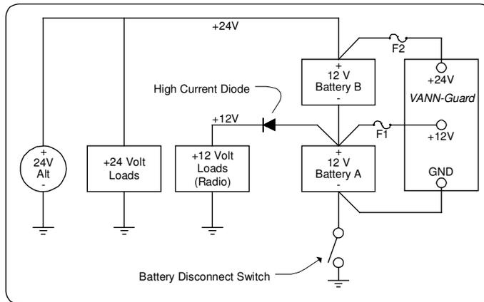
The system must be wired as shown to prevent Reverse Polarity Damage to polarity sensitive 12 volt loads while the ground-side disconnect switch is open. The *VANN-Guards* GND terminal must be wired to the battery side of the ground-side disconnect switch circuit for the *VANN-Guard* to work properly.
