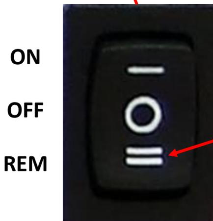
TS Inverter Switch **MUST** be in the **REM** position to function properly.
